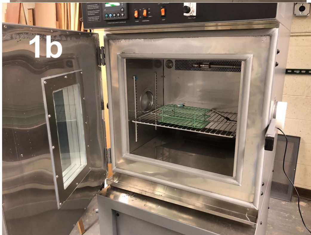
Figure S1. Experimental setup of 2a) a N95 respirator coupon attached to a coated metal rack with metal binder clip and 2b) the rack with a coupon placed in the temperature and humidity-controlled oven.
