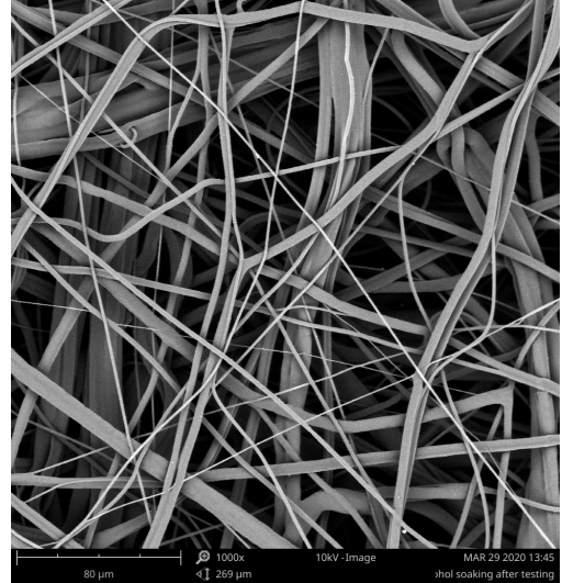
Figure S1. Comparison of fibers before and after alcohol treatment. A. Before treatment, B. after treatment. No differences in morphology, or damages were observed.
