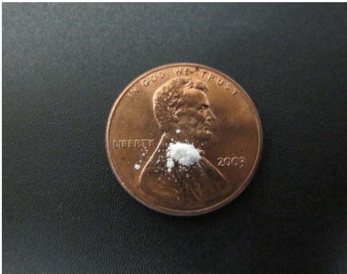
Figure 6: 10 milligram of talc for scale on a U.S. penny. An equivalent amount of the Kelwa Marble Dust as tested would contain approximately 37,000 countable fibrous structures of the regulated asbestos mineral tremolite. Source: Authors.
