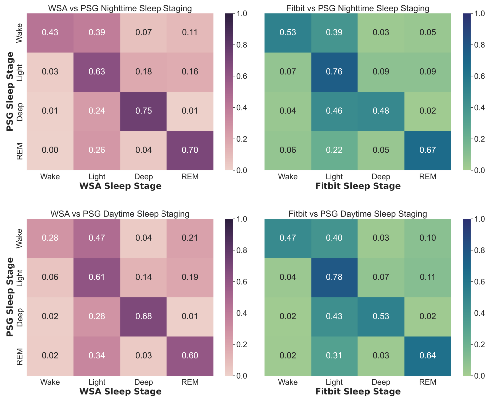
Figure 3: Confusion matrices showing four-stage classification, compared to polysomnography, for Withings Sleep Analyzer versus Fitbit.
