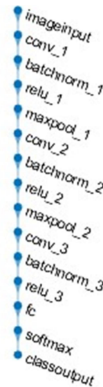
Figure 4. Architecture of the convolutional neural network used.
