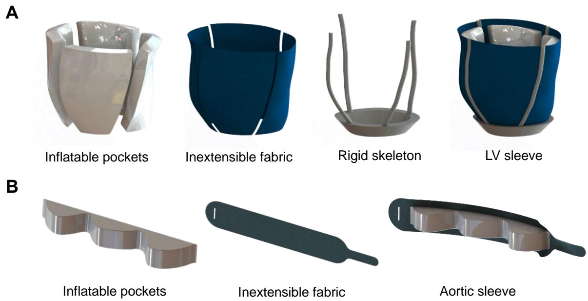
Fig. S2. Design of LV and aortic sleeves. (A) Inflatable TPU pockets, inextensible fabric layer, rigid skeleton, and assembly of the LV sleeve. (B) Inflatable TPU pockets, inextensible fabric, and assembly of the aortic sleeve.
