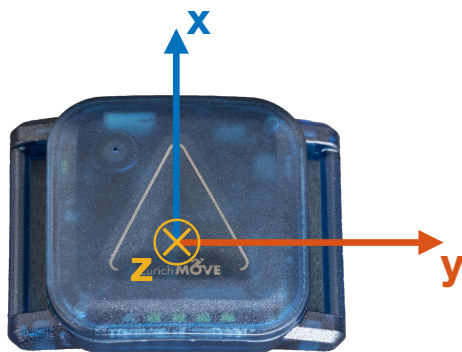
Figure 1: The ZurichMOVE sensor and its coordinate system (created by Rehabilitation Engineering Laboratory, ETH Zurich).
