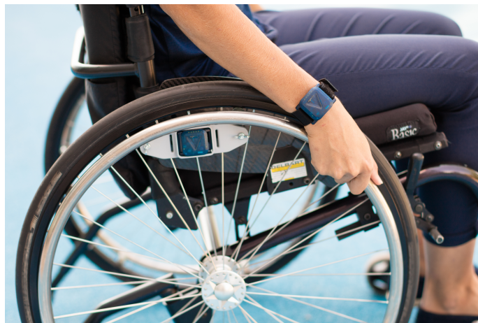
Figure 3: Sensor placement of the wheeling detection algorithm (created by Rehabilitation Engineering Laboratory, ETH Zurich).
