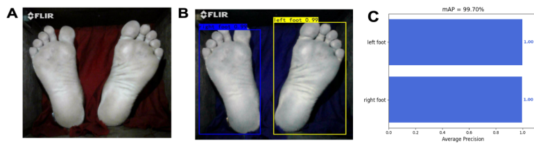
Figure 5: A) Raw Visual Spectrum images B) YOLOv4 predictions on foot presence after training C) AP score of left and right foot
