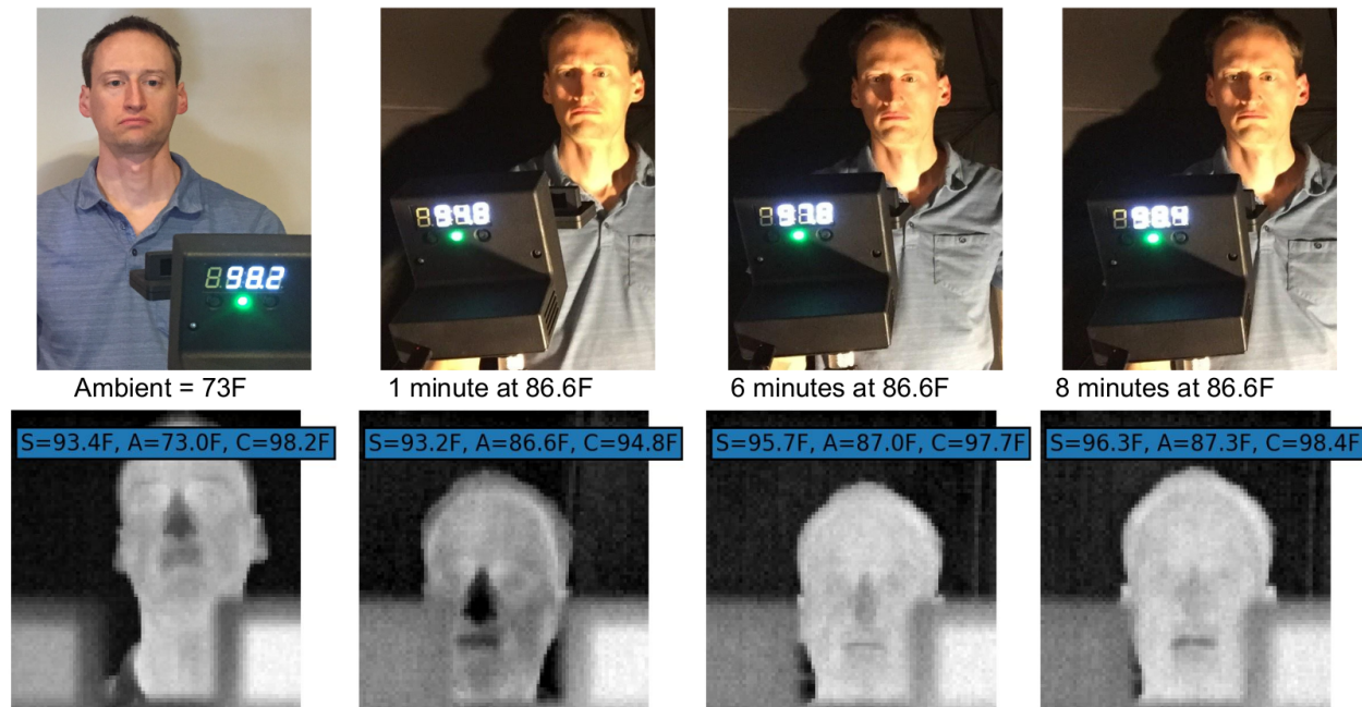
Fig. 6 Exposure to different ambient (A) temperatures adjusts the surface (S) temperature, but may not affect core (C) temperatures. Example of an equilibrated subject moving from one environment (73F) to a warmer environment (86.6F) and the gradual evolution of the surface temperature. Calculation of core temperature based on Eq 1 (using F=0.234 from the pilot study) is correct only when the subject has equilibrated to the environment, as shown in the first and last panels only, with errors shown in the intervening panels.
