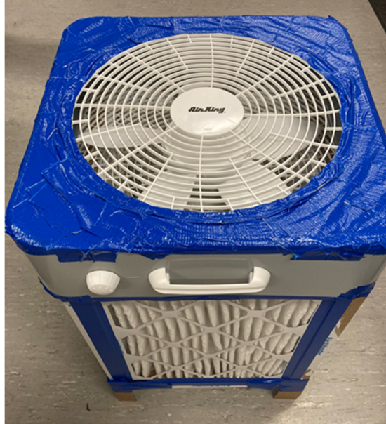
Figure S3. A photo of the assembled Corsi-Rosenthal Box.
