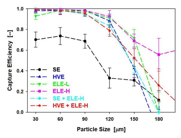
Figure 5. Size dependent capture efficiency of various mitigation device(s) by DIH when cleaning facial surface of teeth #8 & 9. (SE: saliva ejector; HVE: high-volume evacuation; ELE-L: extraoral local extractor at low flow setting; ELE-H: local extractor at high flow setting; '+' denotes a combination of two devices. Error bars represent standard deviations of three measurements.)
