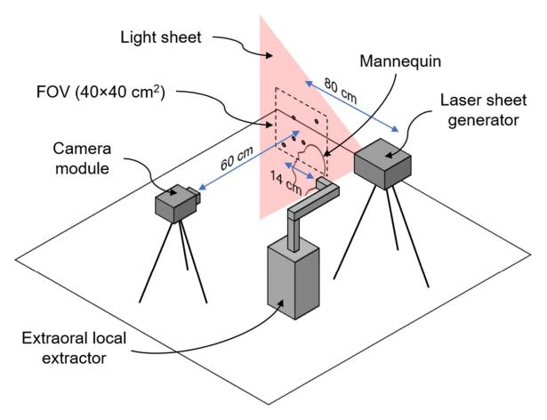
Figure 2. Schematic of LSI setup used for far-field plume and splatter measurements. The camera module incorporates a camera sensor, image intensifier and imaging lens, and the laser sheet generator is composed of a high-power laser and a set of optical lenses. A detailed description of the system can be found in Supplementary Information.
