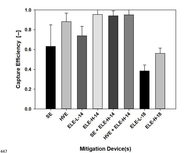
Figure 6. Capture efficiency of various mitigation device(s) by LSI when cleaning facial surface of teeth #8 & 9. (SE: saliva ejector; HVE: high-volume evacuation; ELE-L-#: local extractor at low flow setting at a distance of # cm; ELE-H-#: local extractor at high flow setting at a distance of # cm; '+' denotes a combination of two devices. Error bars represent standard deviations of three measurements.)
