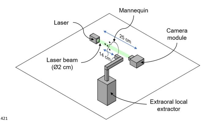
Figure 1. Schematic of DIH setup used for near-field aerosol size and velocity measurements. The DIH system is mounted onto a cage system secured to a table (not shown) and incorporates beam expanding, collimating and condensing optics (also not shown). A detailed description of the system can be found in Supplementary Information.
