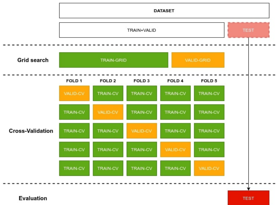
Figure 4: Dataset split of our experimental framework. The size of the train and validation sets is the same for each fold and for the grid search. None of the validation sets used in the CV is the one used in the grid search.
