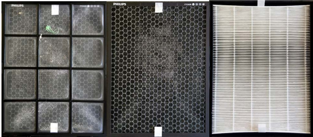
Figure S5: Pre-filter (left), active charcoal filter (middle) after one week of operation in the classroom. Coarse dust, hairs and fluff can be discerned. No deposits of particles could be discerned by eye on the HEPA-Filter (right). Sections that appear darker are due to the illumination.
