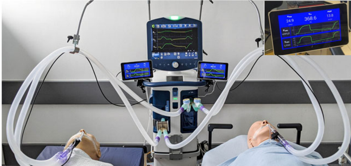
Figure 02. Image of the assembled system attached to two manikins. Monitoring of the respiratory parameters for each limb are shown to the right and left of the main ventilator. A closeup of the display readout is also shown.
