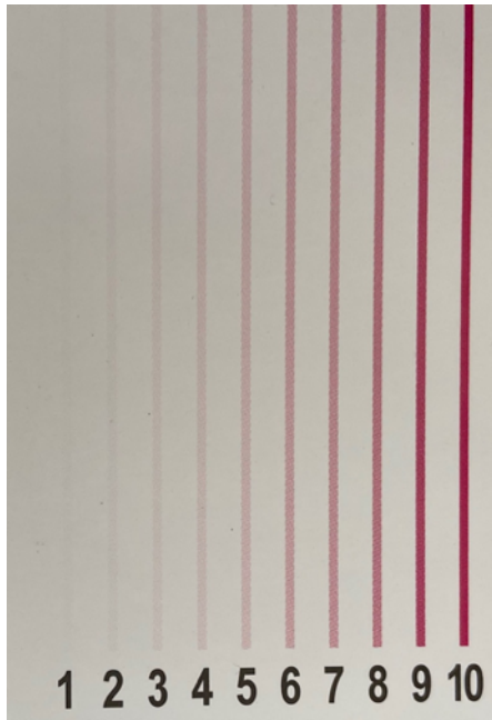
Figure S2: Visual Score card for quantitative interpretation of AbC-19 LFIA test bands. A scale of 0 (not pictured, negative-no test line visible) to 10 (positive-strongest test line). Any LFIA scoring 1 or above was classified as positive.
