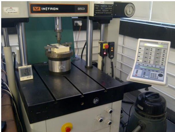
Figure2: Performing pull-out test on a foam block using an Instron 8501 testing machine
