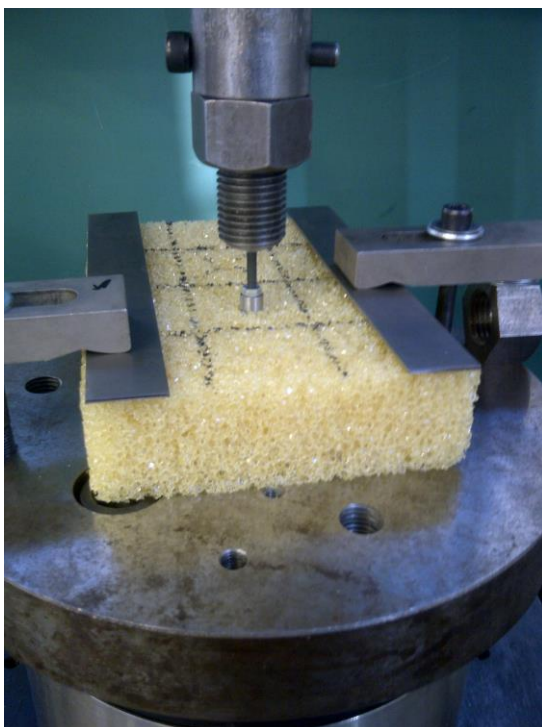
Figure 3: The implant has initialized in the artificial bone block with a density of 0.12 g/cc and ready to start the pull-out experiment.
