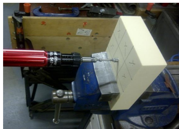
Figure1: The torque required to insert the new implant into the foam block was measured using a torque meter.
