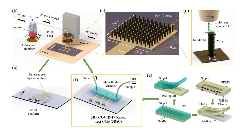
Figure 2. Functionalization of 3D Printed Micropillar Electrode and 3DcC Sensor Operation.
