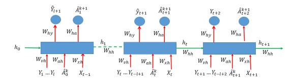
Figure 1. Architecture of RNN encoder.
