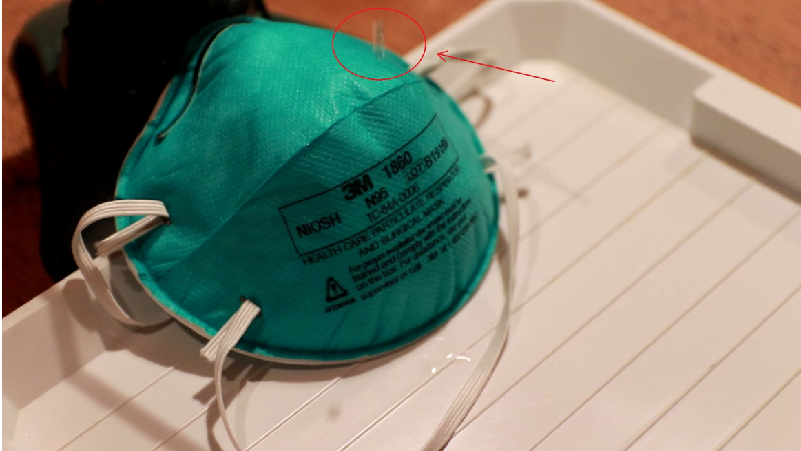
Fig. 4. A sample frame of the video capture of the fluid resistance validation test, showing the water droplet prior to encountering the hydrophobic layer of the mask surface.
