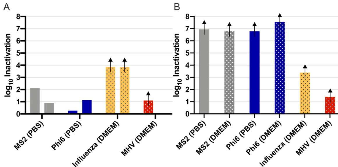
**Figure 1.** Virus removal from pulsed xenon UV followed by 82 °C heat for 30 mins. (A) Heat treatment with low relative humidity (~8% RH) and (B) heat treatment with moderate humidity (62-66% RH at 80 °C). Each bar represents the average of replicate experiments conducted on a single day (n = 2-3). Arrows identify samples that exceeded assay detection limits after treatment. Viruses were deposited on the coupons in either PBS or DMEM culture medium.
