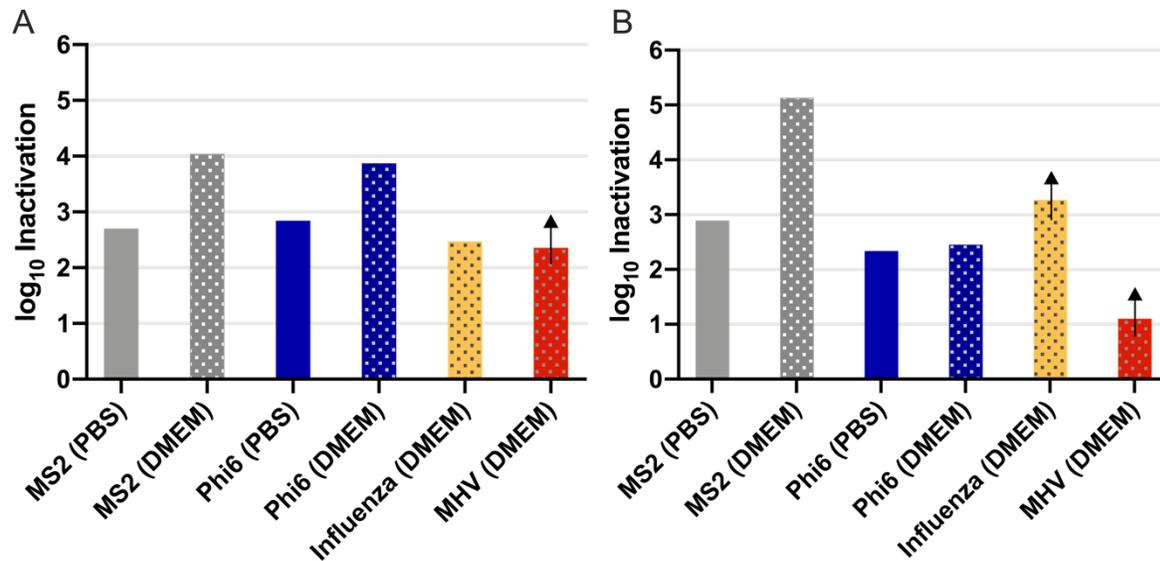
**Figure 2.** Virus removal from Bioquell VHP system with either A) Condition 1 and B) Condition 2. Each bar represents the average of replicate experiments conducted on a single day ( $n = 2-3$ ). Solid bars represent experiments where viruses were deposited in PBS and textured bars represent data where viruses were deposited in DMEM. Arrows illustrate samples that exceeded assay detection limits after treatment.
