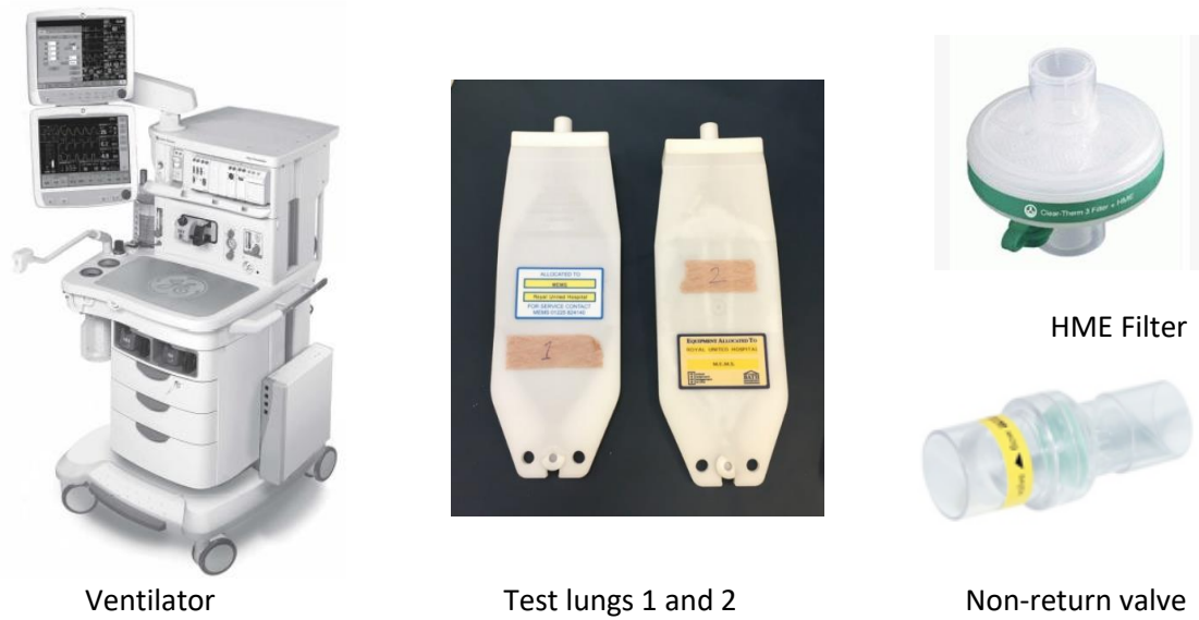
Figure 2. Test system components (with acknowledgement to GE Healthcare and Intersurgical)
