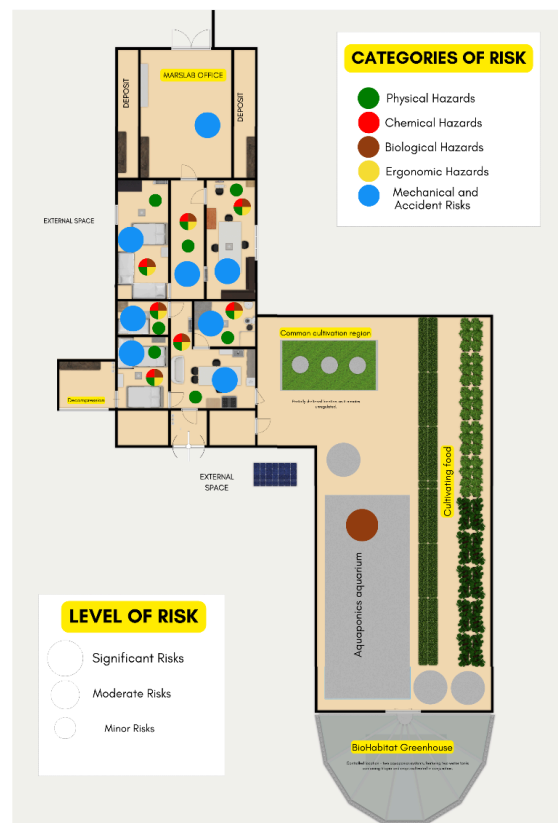
Fig. 6. Risk map of the base of the Habitat Marte analogue station. Source: Author's own elaboration.
