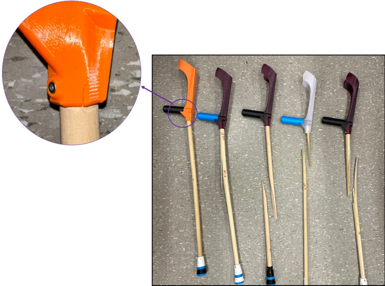
Figure 11. failure points for each of the 2 types of failure.
