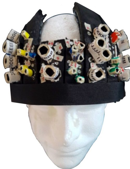
107 108 Figure 1. Picture of the helmet. The design features an open area at the top of the skull to avoid interference 109 with invasive neuromonitoring devices.
