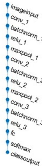
Figure 4. Architecture of the convolutional neural network used.
