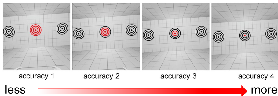
FIG. 4: Illustration of the accuracy parameter, ranging from 1 (low accuracy, the whole target is the validation zone) to 4 (high accuracy, the central disk is the validation zone).
