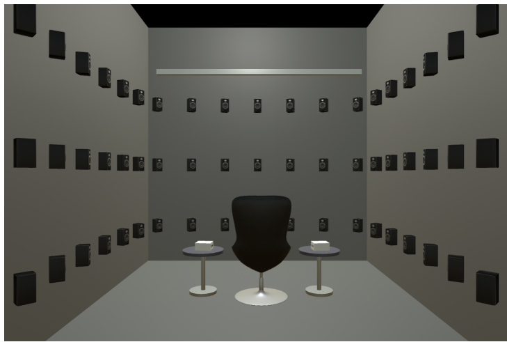
Figure 1. Auditory 3D motion localization : condition A1. a) Experimental set-up with 97 speakers on the walls & on the ceiling; b) Group scores in bilateral cochlear implant users (BiCI) in comparison to the typically hearing individuals; scores of other hearing device users (other CI/HA) represented as individual crosses on the right side. Statistical comparisons with a Wilcoxon signed-ranks test (***) p < 0.001 , ** p < 0.01 , * p < 0.05 ). Data are represented as mean \pm SD.
