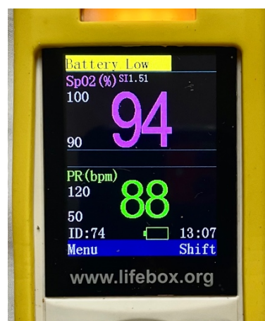
Figure 3. Images of the first version of the family member observation chart and the pulse oximeter used, illustrating the discrepancy between positioning of heart rate (bottom, in green on the pulse oximeter) and oxygen level (top, in pink on the pulse oximeter)
