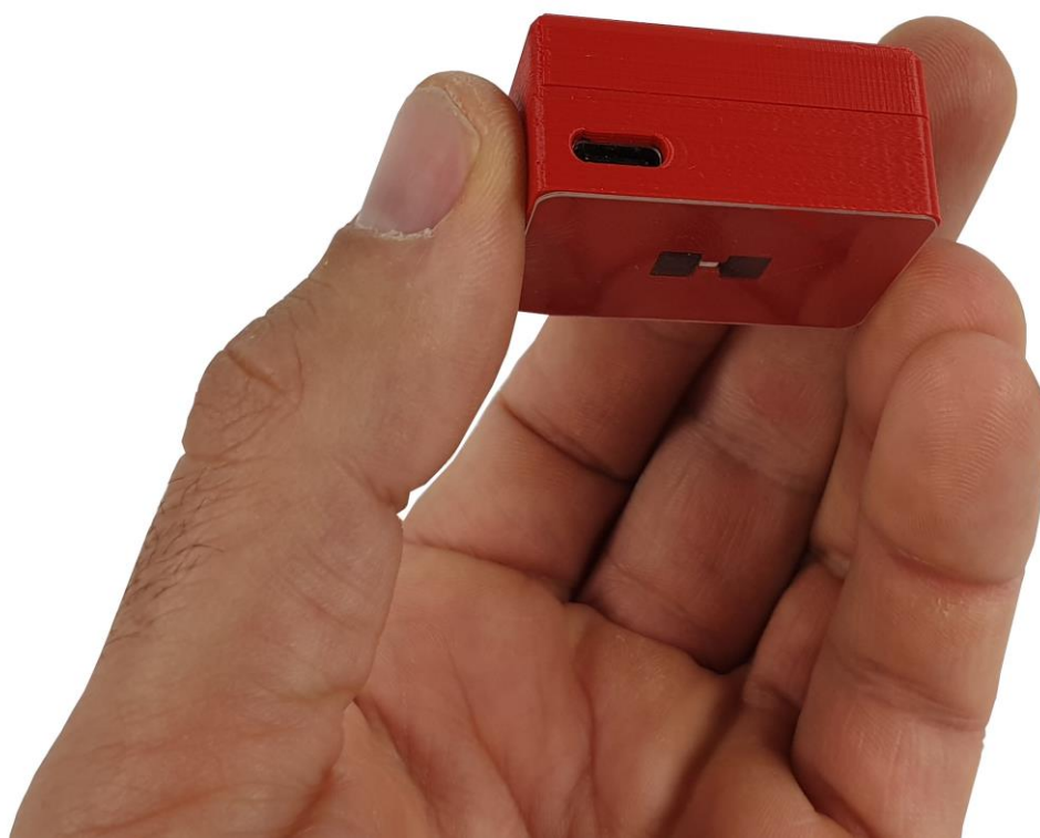
Figure 1. Picture of the penile self-developed sensor (measuring 41 x 27 x 19 mm)
