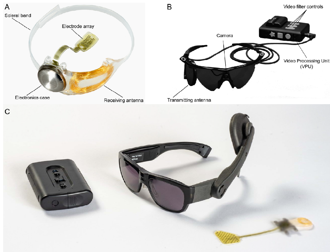
Figure 1: Overview of the Argus II (A-B, reused under CC BY-NC-ND from Ref. 22 ) and Orion implants (C, https://cortigent.com ). (A) The implanted components of the Argus II system include a hermetically sealed enclosure for the electronics that, along with a receiving antenna, is secured to the eye with a scleral band and sutures, and an array of 60 electrodes that is inserted into the eye and tacked over the macula. (B) External (body-worn) components of the Argus II system include a pair of glasses with a small camera mounted in the frame connected via a cable to a video processing unit (VPU) worn on the belt or on a shoulder strap. (C) This future depiction of the Orion device includes an external data processing unit, which deciphers visual inputs relayed from a
