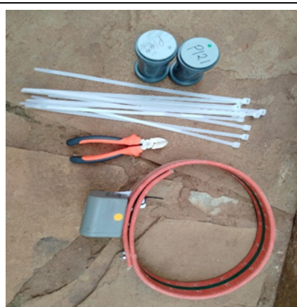
347 348 349 350 351 352 353 354 355 Figure 4: CatLog2 GPS logger (top) and Savannah GPS logger (bottom), with the items used for affixing the loggers.
