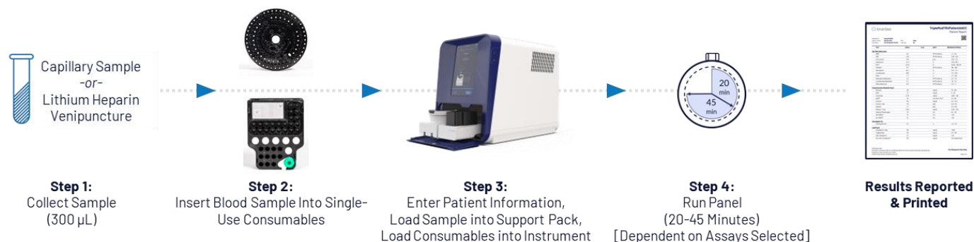
Figure 2. The Truvian platform is fully integrated and automated with no upfront processing or pipetting steps required. Step 1: Collect minimum 300 µL whole blood sample, Step 2: Insert the sample (300 µL tube of Li-Hep blood) into the Support Pack, Step 3: Enter patient information and place single-use Disc and Support Pack into the device, Step 4: Start the panel. At the end of the run, panel results are displayed on the device and can be printed. The consumables are then ejected to be disposed.
