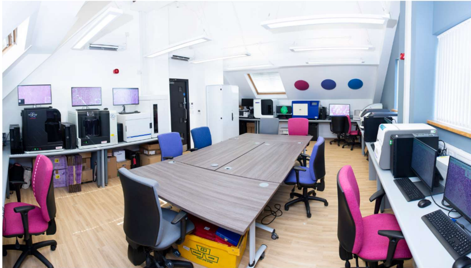
Figure 5. NPIC AI FORGE post installation image. Image shows the FORGE layout with a central island of tables for the receipt, preparation, and post scanning activity of glass slides with a quick access slide cabinet less than 1 meter away. Scanners are spaced with sufficient access allowance. Operator workstations are positioned throughout the facility and all monitors are high grade, manufacturer provisioned, or NPIC sourced medical grade displays. Sufficient lighting and air-conditioning capacity can also be seen.
