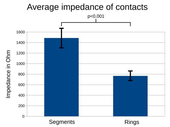
**Figure 4:** Average impedance of contacts. The impedance of segmented contacts was twice as high as for ring contacts, thus necessitating a higher energy delivery when the same stimulation parameters were applied.
