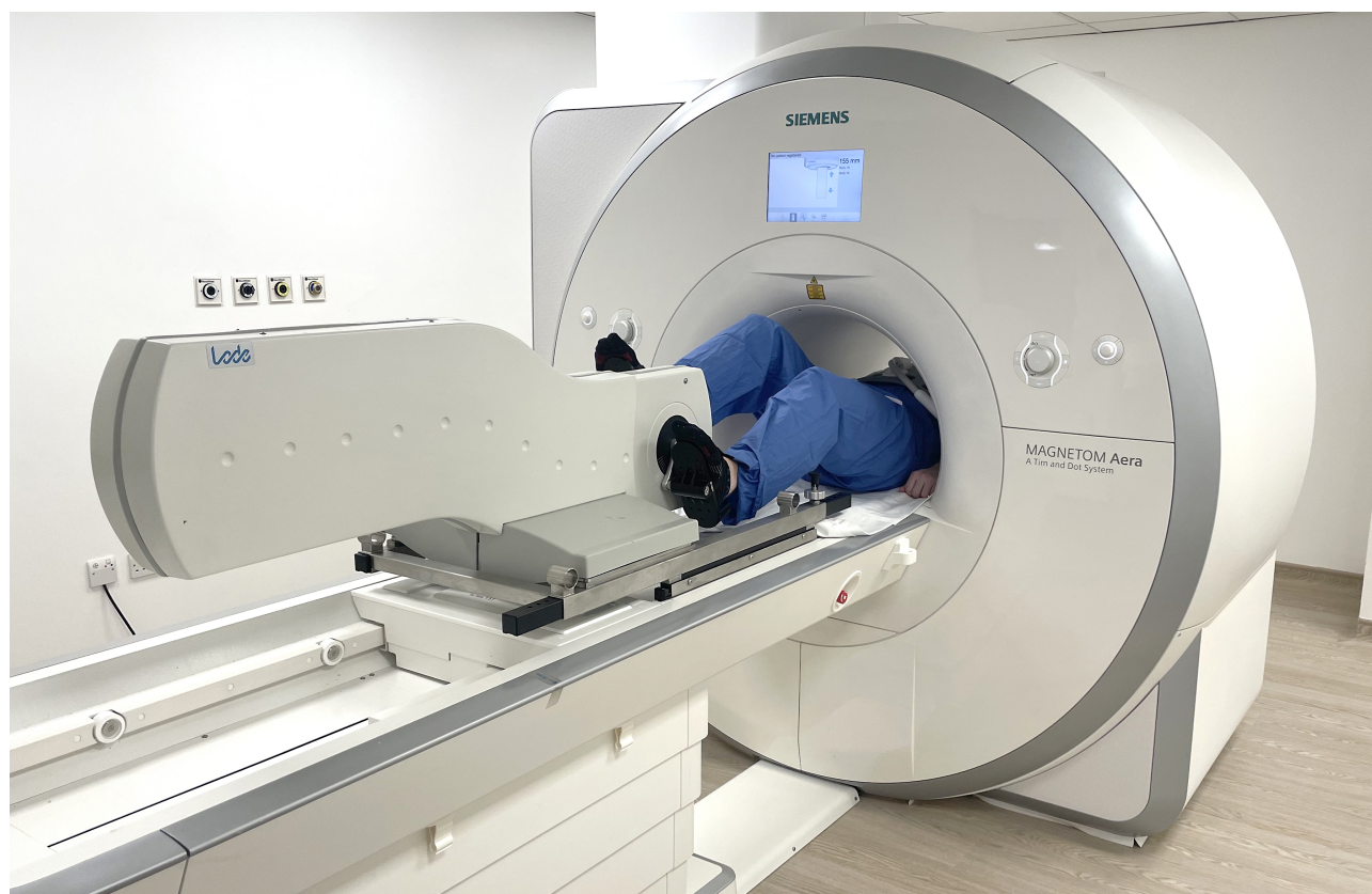
Figure 2. Pedal ergometer. Positioning of the bed-mounted MR-conditional pedal ergometer allowing participants to exercise while at isocentre (hand holds not shown). An electro-magnetic braking system allows a maximum peak load of up to 300W. An external control unit displays multiple ergometry parameters in real time.
