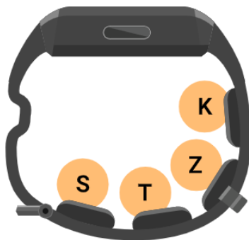
Figure 1. The Neosensory wristband has four vibrating motors embedded in the wrist strap. The top of the wristband contains a power button and a microphone. Each phoneme is assigned to an independent motor.
