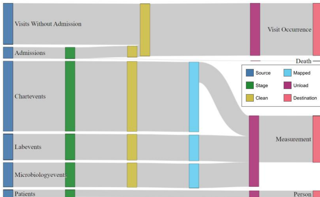
Figure 2: The figure illustrates the data flow diagram of four different entities. In all cases, the data from the source schema is imported into a staging table which is transformed into standard entities after performing cleaning and mapping to a desired standard. The standard entities are dumped in the unloading table which will be finally pushed to the destination OMOP-CDM schema.
