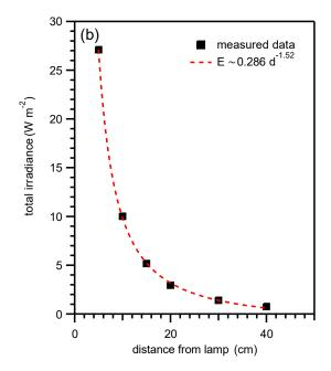
**Figure 1.** (a) GUV222 lamp emission spectra showing peak emission at 222 nm measured at six different distances. (b) The total irradiance versus distance showing a drop-off proportional to  $1/d^{1.52}$ .
