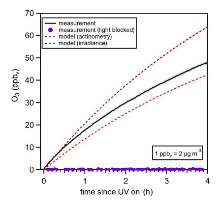
**Figure 2.** The average  $O_3$  mixing ratio from seven GUV222 lamp experiments is shown as the solid black line with the variability ( $2\sigma$ ) shown by the gray shaded area. The average and standard deviation of seven modeled  $O_3$  mixing ratios is shown as determined by the irradiance method in dark red and actinometry method in light red. The  $O_3$  measured from the experiment where the light was blocked is shown in purple.
