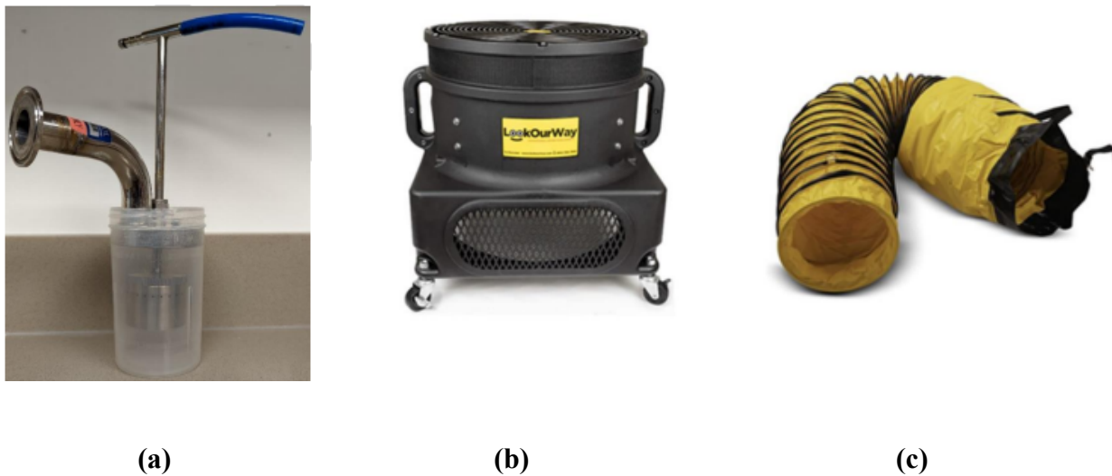
Figure 26. Materials used in test space: (a) 24-jet Collison nebulizer with 304 stainless steel construction (BGI Industries). (b) The 1HP blower used to move air within the test chamber. (c) The 18" diameter flexible duct used to bring in fresh air through the inlet.
