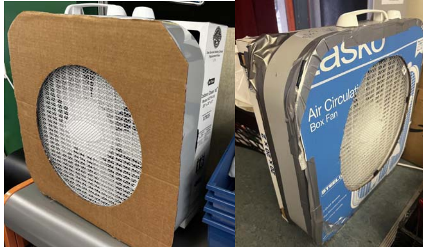
Figure 3: DIY air purifiers made from Lasko fans and 5” Lennox MERV 16 (left) and 2” Nordic Pure MERV 13 (right)
