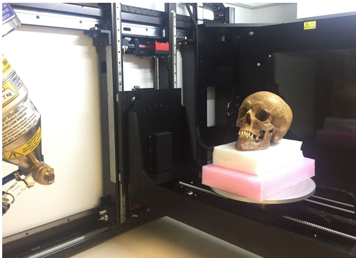
Figure 1. Large Volume Micro-CT. Sample SMB73 - adult male (age 35 - 45 years). Showing the entire skull in position before scanning using the Nikon XH T 225 ST cabinet style system (15).
