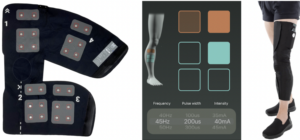
Fig. 2. . Left: Cionic Neural Sleeve showing the configuration of the FES and EMG electrode arrays. Center: Cionic mobile application interface for setting FES parameters (frequency, pulsewidth, intensity) and current field steering. Right: Cionic Neural Sleeve on body.
