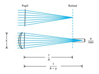
Figure 1 The optical model of minimum limit of discernible change in spherical power
