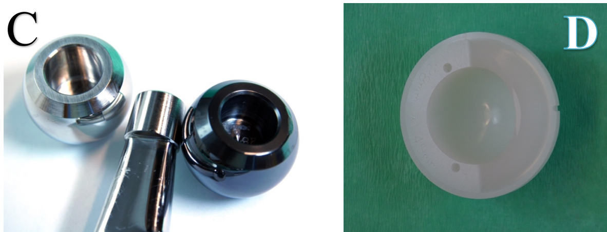
Figure 2. C. CoCrMo 28 mm femoral head (left) and Oxinium 28 mm femoral head (right). Spectron EF stem taper (middle). D. Reflection All-Poly UHMWPE cup
