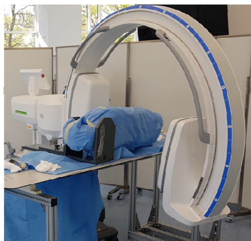
Fig. 1 Experimental setup with specimen and mobile C-arm and visualization of the degrees of freedom investigated.
