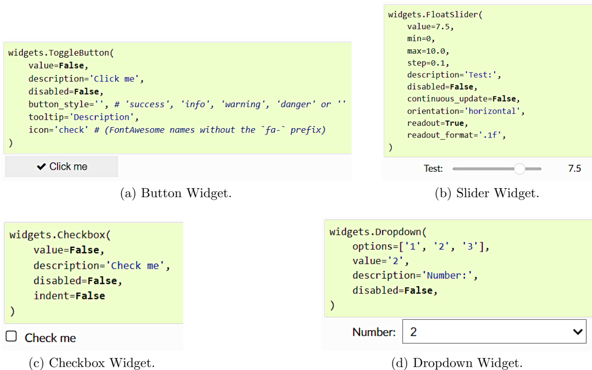
Figure 4: Illustrations of some of the Widgets from the iPywidgets module used in the app
