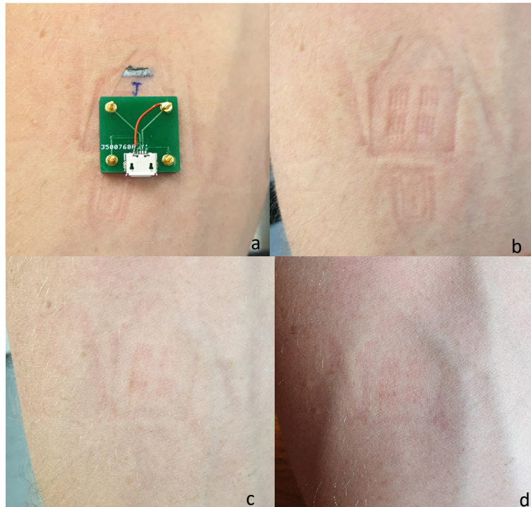
Figure 6 – photographs showing: a) lactate biosensor in situ on participant forearm without connecting wires; b) underlying skin after immediate removal of biosensor; c) underlying skin after 15 minutes of biosensor removal; d) underlying skin after 60 minutes of biosensor removal
