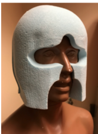
Fig. S1. Caseforge head mold on KEMAR acoustic research manikin.
