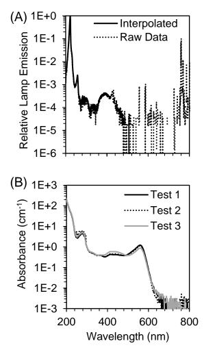
**Figure S1:** (A) The raw spectral emission from 200 - 300 nm of the filtered excilamp (USHIO Care222®) was interpolated and relativized to the peak emission at 222 nm for use in UV dose calculations and plotted on log scale to show orders of magnitude less but non-zero emission at filtered wavelengths > 240 nm. (B) The absorbance spectrum from 200 - 300 nm of SARS-CoV-2 at ~10<sup>5</sup> PFU/mL in cDMEM was measured for each of three Tests for use in UV dose calculations.
