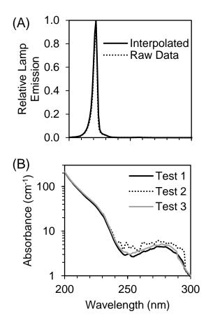
**Figure 1:** (A) The raw spectral emission from 200 - 300 nm of the filtered KrCl excilamp (USHIO Care222®) was interpolated and relativized to the peak emission at 222 nm for use in UV dose calculations. (B) The absorbance spectrum from 200 - 300 nm of SARS-CoV-2 at ~10<sup>5</sup> PFU/mL in cDMEM was measured for each of three biologically independent Tests for use in UV dose calculations. Expanded emission and absorbance spectra from 200 - 800 nm are shown in Supplementary Figure S1.
