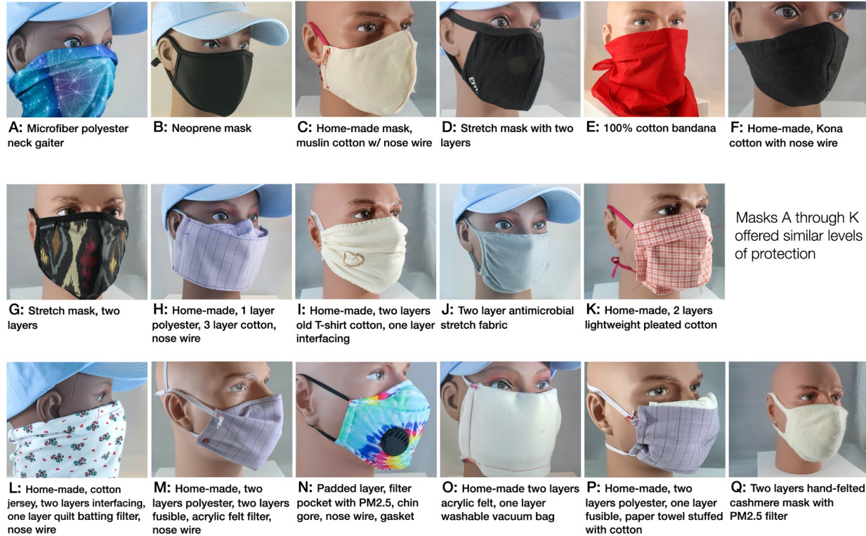
Fig 1: Photographs of the seventeen masks assessed for their protection factor on mannequin heads. Details of the construction and materials of each mask are included whenever possible. Masks that were home-made are identified.
